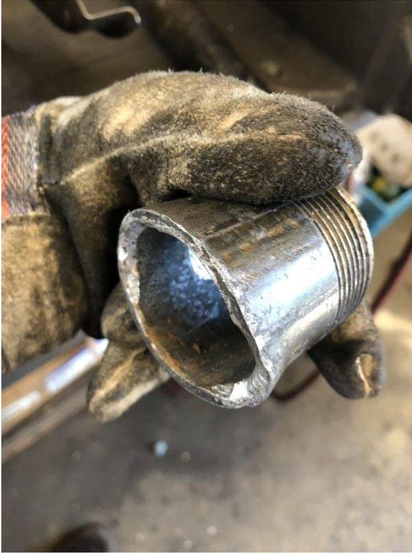
The ductile pipe distorted itself to conform to the A-arm
