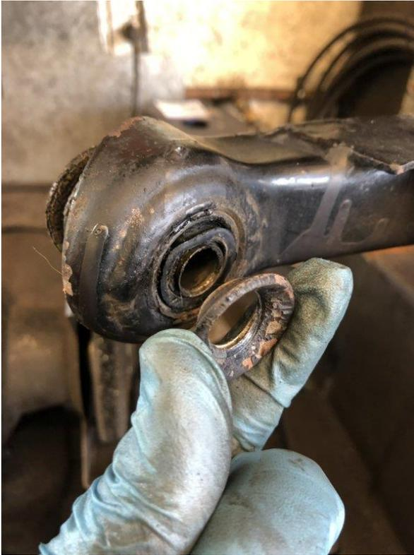
Destroying the bushing washer to achieve 'steel-to-steel' contact
