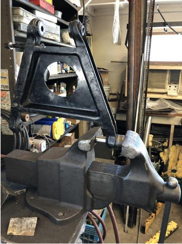
Typical situation at the bench vice.. That's the lower A-arm with a 7/8" socket on the "pushing" side and a piece of ductile iron on the other, "receiving" end
