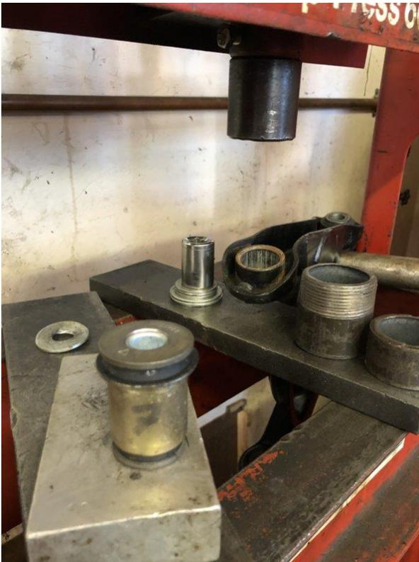
Typical situation at the press - using pipes and sockets
