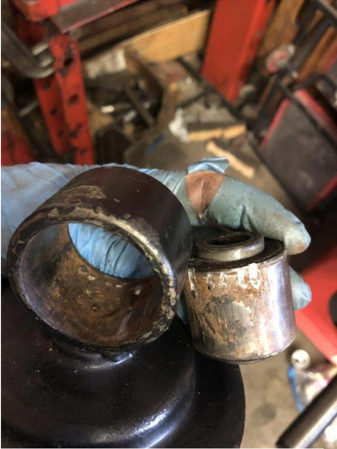
The welding snots inside the Upper Shock bore
