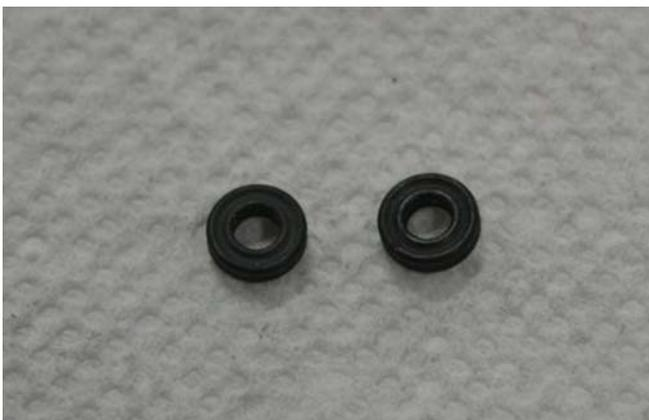
If you feel the cylinder itself is the cause of the leakage I would still encourage you to try replacing the port seals first. As I said before, it is many times difficult to determine the cause of the leak and all three of the Khamsin leaks were fixed by replacing the port seals.
