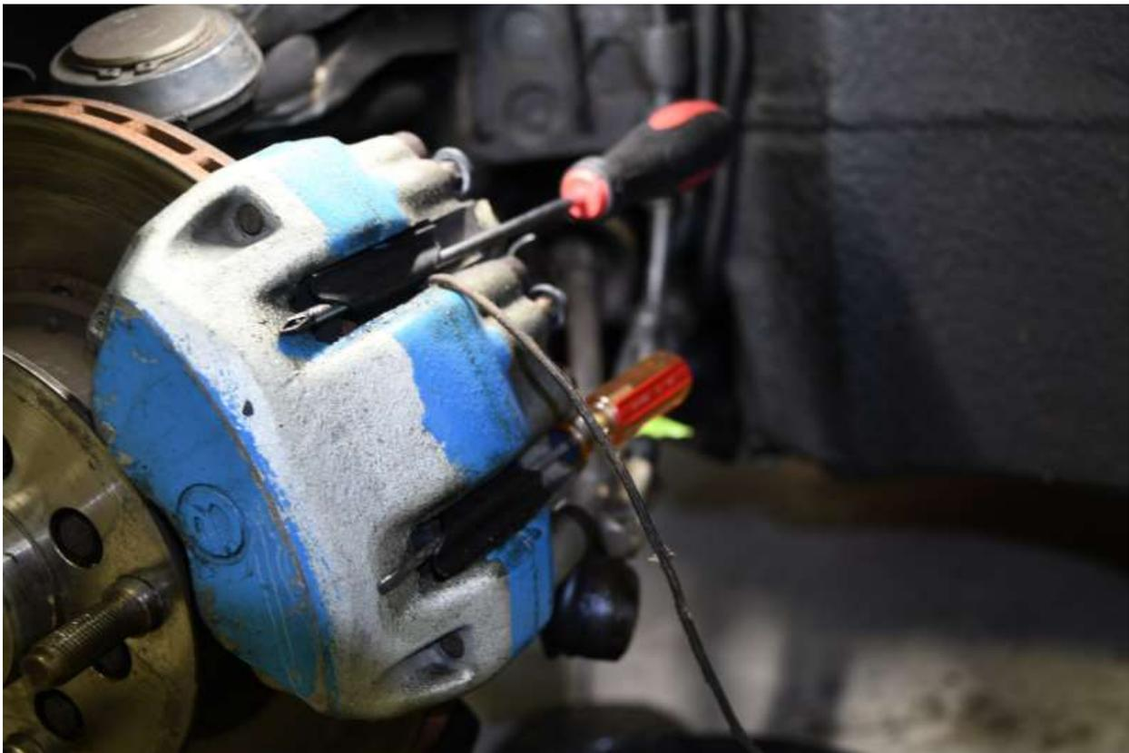
5. Use a 19mm socket to remove the two bolts holding the caliper. Remove the caliper from the car.
