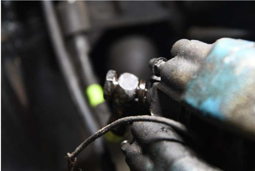
4. Use two screwdrivers to hold the anti-rattle plate in place. This is an important step as it will make removal and insertion of the pads possible. I did not make up this step as the same calipers are used on the Detomaso Pantera and the factory service manual for that car specifies this step. I tried to insert the pads without the screwdrivers and failed.
