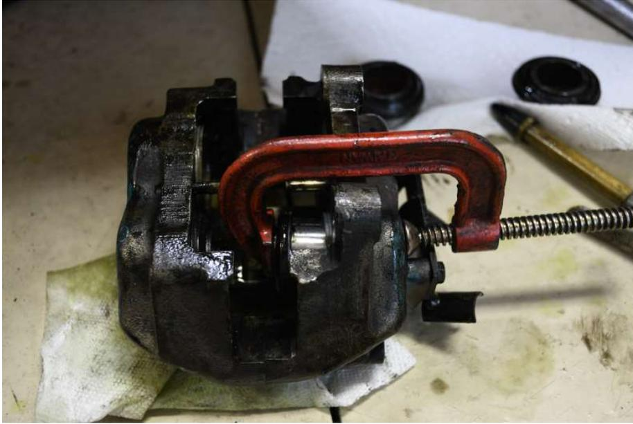
8. Remove the old piston seals from inside the bore.
