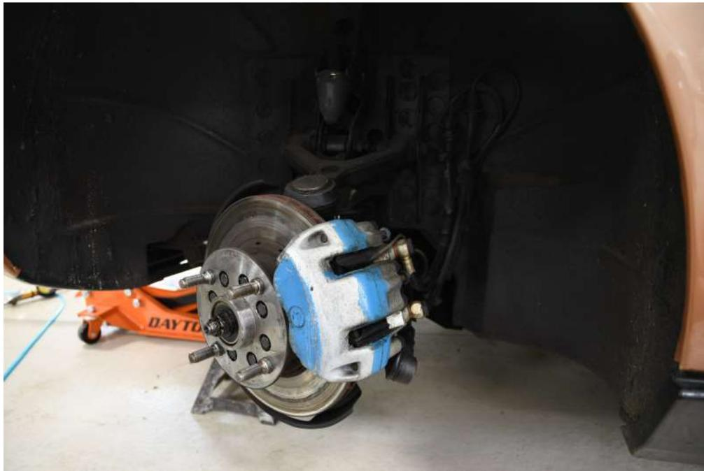
1. Disconnect the brake pad electric wear sensor wire (if there is one on your car)
