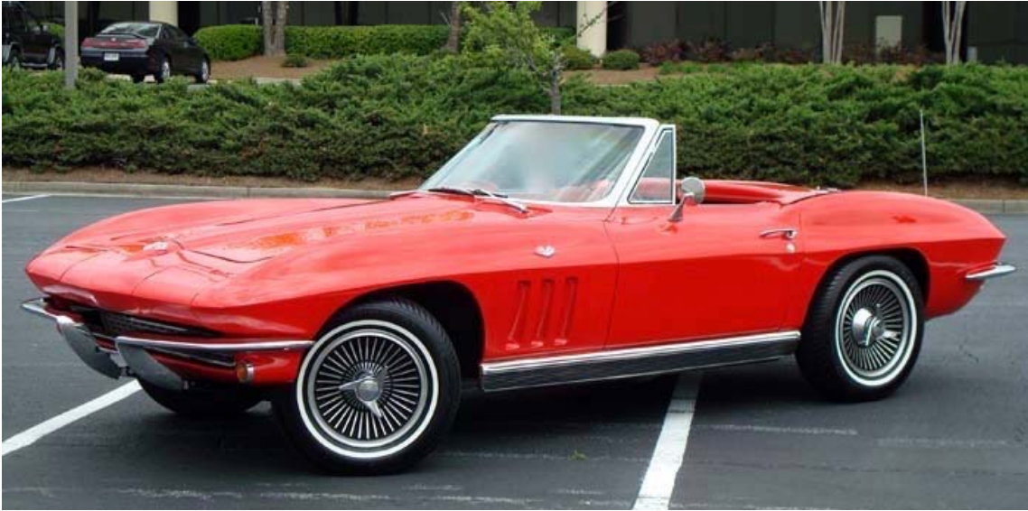
1966 Corvette: Wheelbase 98"; Length 175"; Width 70"; Height 50"; Weight 3,250 lbs
