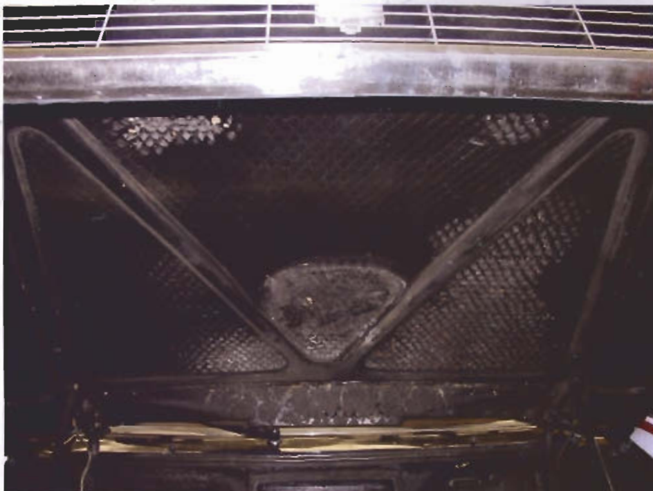
Carburetor fire damage.
